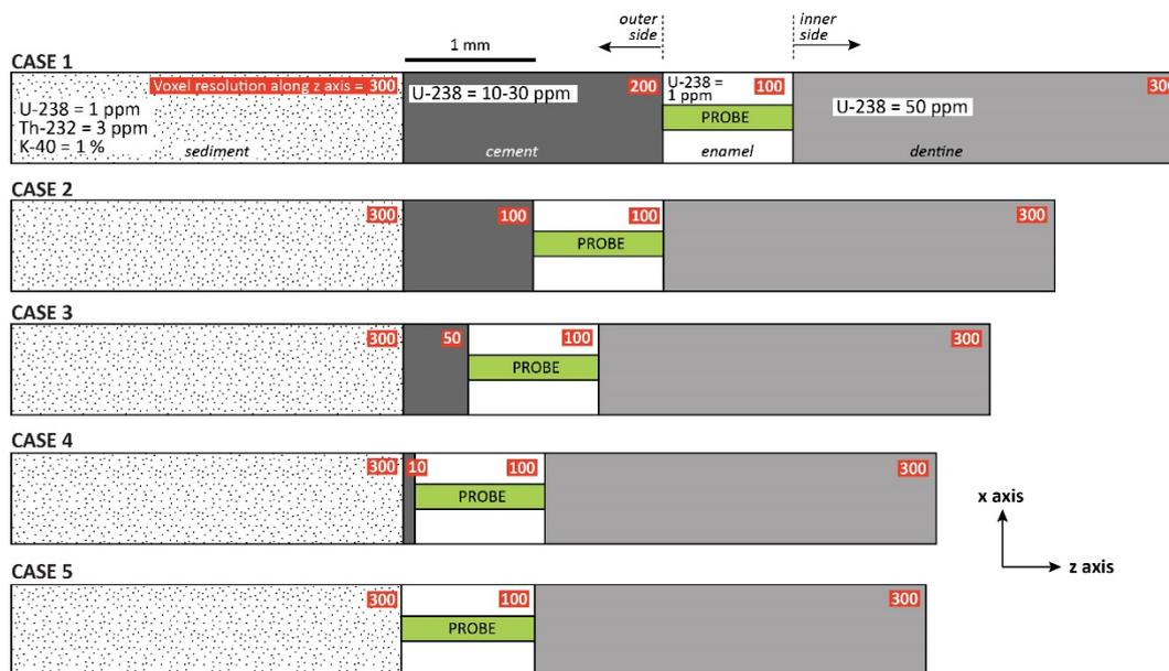
Fig. 2. 2D schematic display of the 5 cases simulated with DosiVox (along  $z$  axis). The number of voxels used for each component along the  $z$ -axis is indicated in the red boxes. Note that a  $1 \times 1$  voxel of  $20 \times 20$  mm was considered in the  $x$ - $y$  plan for the simulations. Simulations were performed by considering 10, 20 and 30 ppm of U-238 in the cement.
