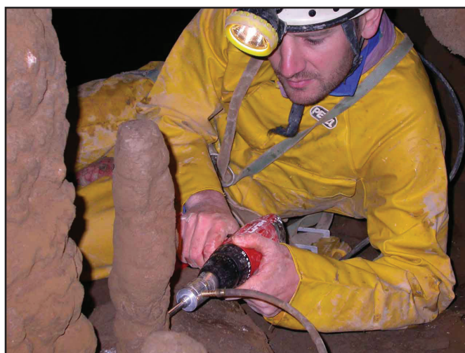
Fig. 5. A light-weight battery-powered drill is used in conjunction with a water-flushed drill to obtain small cores from the inner part of stalagmites for a rapid screening a large number of speleothems.
