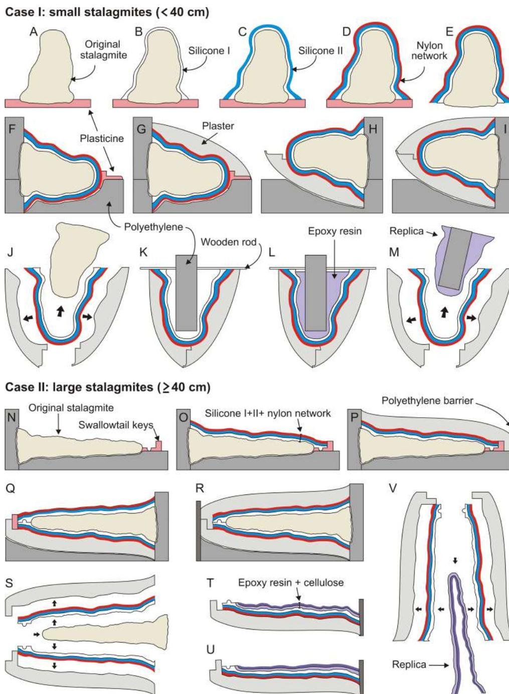
Fig. 3. Molding and casting scheme for stalagmites. See description in text.
